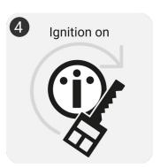
The IOPEDAL automatically starts the Auto-Ranging mode during initial startup (ignition on/engine running). In this mode, the system analyzes the signals from your accelerator pedal throughout its entire travel range and adjusts all driving modes in real time to match your vehicle's characteristics.
